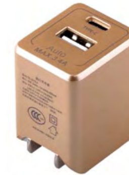
LM05-2452 Travel Charger :Type C & USB 2.0 Input : 100~240V AC 50/60 Hz 500mA Output: TYPE-C:5V/3A(Max),USB:5V/2.4A(Max) Total 5V/3.4A(Max)
