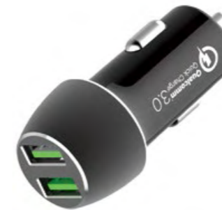
LM05-2354 Car Charger :QC3.0 2Ports Input : 12-24V DC Output: 36W (3.6V-6.5V) 3A,(6.5V-9V)2A,(9V-12V)1.5A
