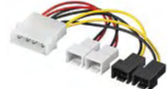
LM01-113406 PC Power 4Pin Male to Female
